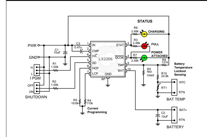
Figure 1 - LX2206 Evaluation Board Schematic
